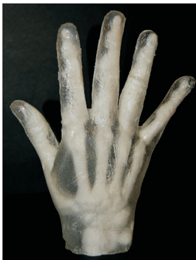
Fig. 8. 3D printed model showing the skeletal structure (white) and the musculature (transparent). The template was made using a computed tomography bone scan and 3D hand scan and printed by dual extruder printing. Model organs can also be printed for students and practitioners.
