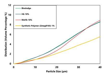
**Figure 4.** Particle size distribution of raw biosludge and conditioned biosludge with 10% of hemoglobin and methylated hemoglobin within the range of 0–40  $\mu$ m.
