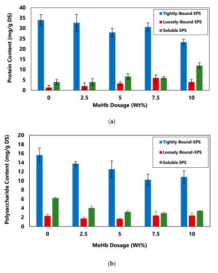
**Figure 6.** (a) Protein content and (b) polysaccharide content of EPS in biosludge at different dosage of methylated hemoglobin.
