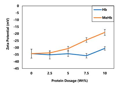
Figure 5. Zeta potential measurement of conditioned sludge with hemoglobin and methylated hemoglobin.
