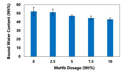
Figure 7. Bound water content in biosludge at different dosage of methylated hemoglobin.
