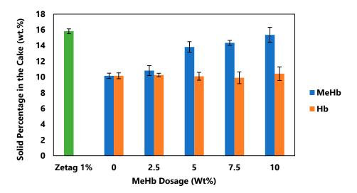
**Figure 2.** Effect of hemoglobin and methylated hemoglobin on cake dry solids content at different dosages.
