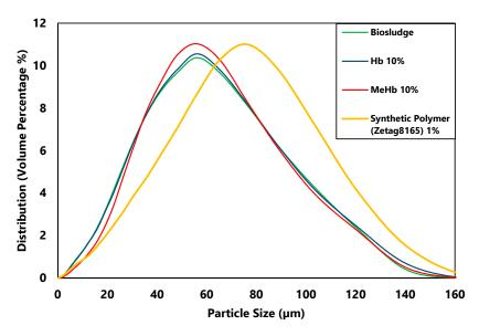
**Figure 3.** Particle size distribution of raw biosludge, conditioned biosludge with 10% of hemoglobin and methylated hemoglobin.
