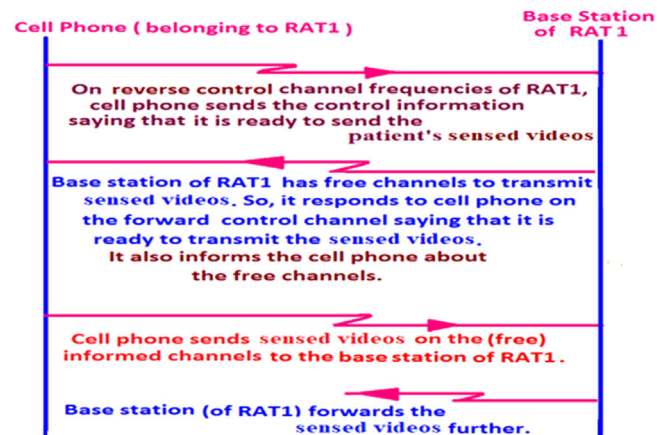
FIGURE 4 Flow diagram for patients' data transmission when cellular network (or RAT1) has enough free channels
