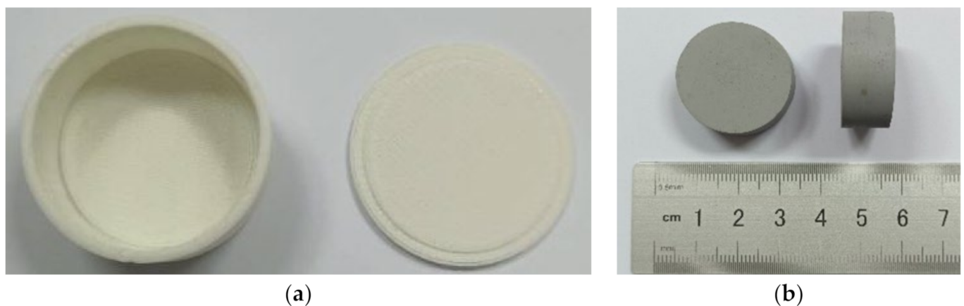
Figure 8. Fabrication of specimen: (a) mold for fabricating specimen; (b) specimen.
