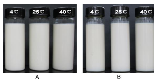
Figure 3. Photographs of Pu-NSSPE (A) freshly prepared and (B) stored at 4, 25, and 40 °C for 6 months.
