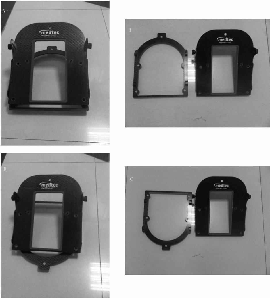
Figure 2 Ready adjustable angle holder reconstructed by us. (A) The adjustable angle holder. (B) The carbon fiber base plate at the bottom of the holder was detached by removing the 4 screws on the bottom. (C) The carbon fiber base plate was reversed. (D) The adjustable angle holder was reassembled.
