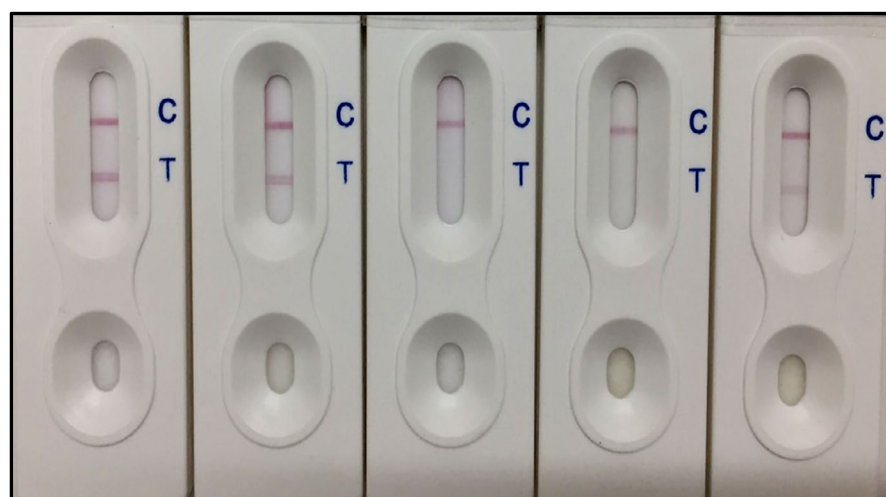
FIGURE 2 Test strips tested with different samples: (A) Phosphate buffer saline (negative control), (B) Urine without albumin (negative control), (C) Human serum albumin (positive control), (D) CKD with urine sample (positive), and (E) Healthy urine sample (negative). C, control line; T, test line
