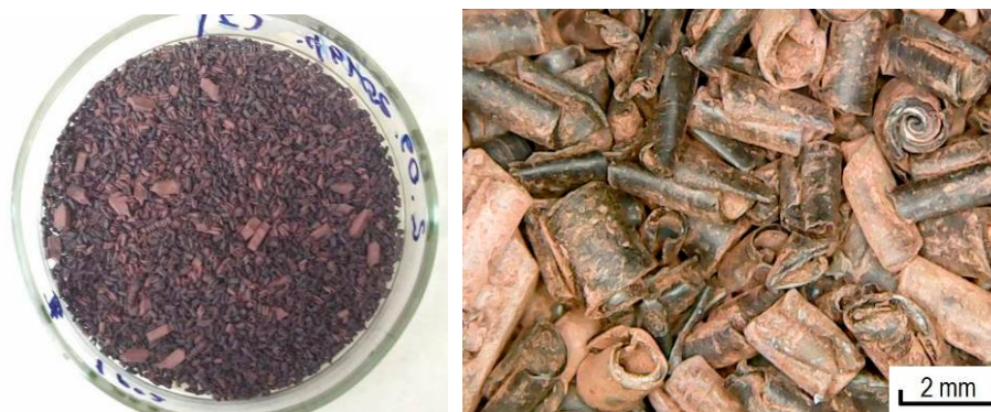
Figure 4. Photomicrographs of copper polypropylene waste.
