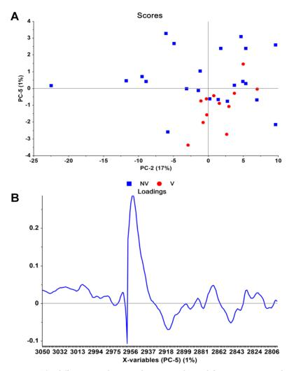
**Figure 3.** The differentiation between the serums obtained from non-vaccinated (NV) and vaccinated (V) individuals by unsupervised PCA. (A) Scores and (B) loadings plot were obtained in  $3050-2800 \text{ cm}^{-1}$  spectral region for NV and V groups.
