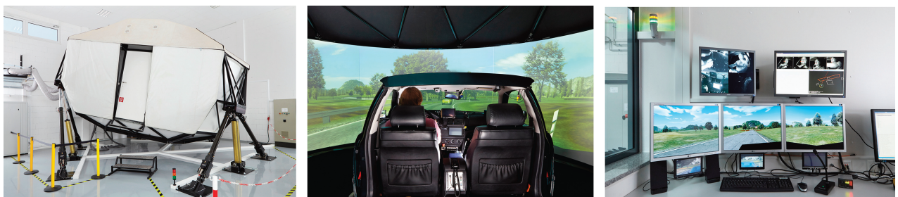
FIGURE 1. The driving simulator of the Würzburg Institute of Traffic Sciences with motion system. The motion system (left) has 6 degrees of freedom. The visual system has 3 image channels that have a field of view of 60 degrees. The environment is also shown in the outside mirrors and the rearview mirror via liquid crystal display. The mock-up (middle) is a truncated BMW series 5. Simulation is operated from a separate room (right). During driving sessions, drivers, their behavior, and the simulated environment can be observed via several monitors (on the right side) and driving errors can be registered without disturbing the driver.
