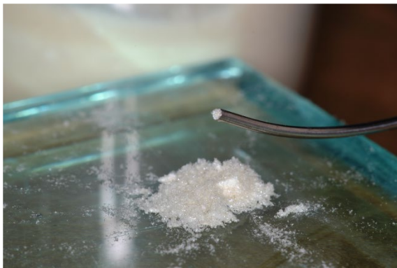
Figure 1. The sericin powder on a glass plate and Angelus MTA applicator of 0.6 mm in diameter can be seen
