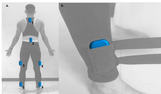
**Figure 2.** IMU device's setting (a) 1: T<sub>2</sub>–T<sub>4</sub>, 2: L<sub>1</sub>–L<sub>3</sub>, 3: VL<sub>left</sub> and 4: VL<sub>right</sub> vastus lateralis, 5: MP<sub>left</sub> and 6: MP<sub>right</sub> malleolus peroneus; (b). body attachment anti-vibration straps system.
