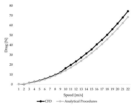
Figure 2. Drag values across different speeds as measured using CFD and analytical procedures.
