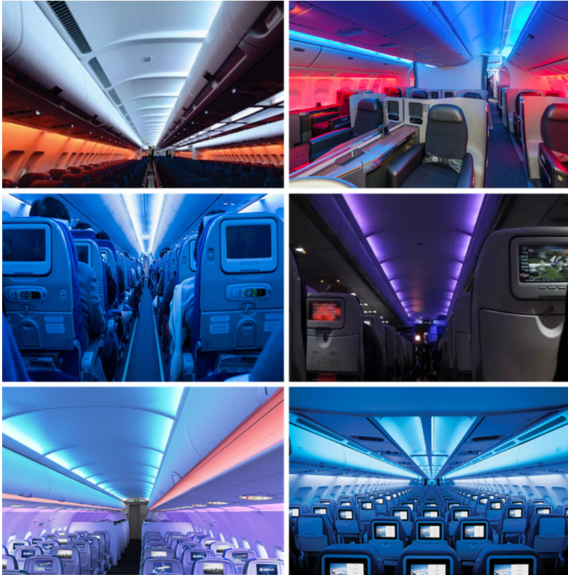
Figure 10.4 Color tunable aircraft cabin-lighting.
