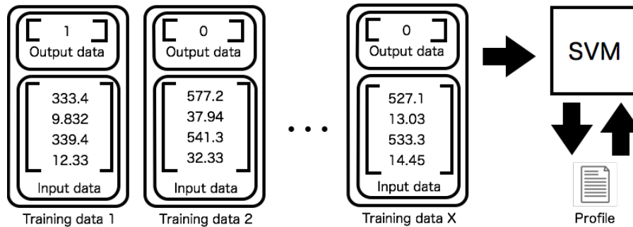
Figure 3. Training process of a profile between two sensors. The training data set are input to an SVM. The SVM learns desired outputs from the training data set.
