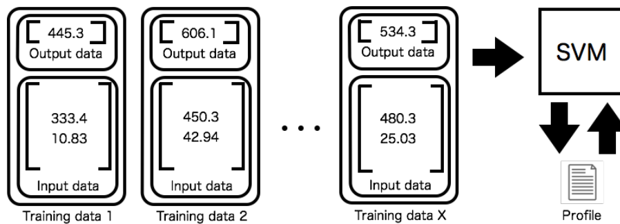
Figure 4. Training process of a profile between two sensors for spatiotemporal interpolation of missing data. The training data consisting of tuple data set are input to an SVM. The SVM learns desired outputs (interpolated value) from the training data set. This profile is used for interpolation. On the other hand, the profile shown in Figure 3 is used for evaluating relations between two sensors.
