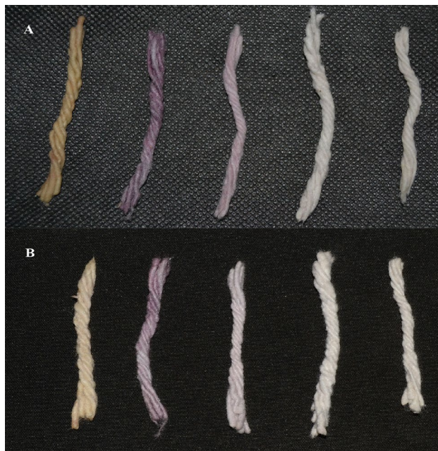
Figure 9. (A) cotton material dyed using gold nanoparticle colloid solution, (B) cotton material after exposure to various stress conditions.
