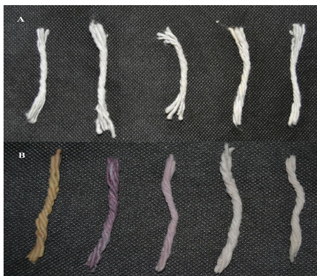
Figure 8. (A) cotton material before dyeing, (B) cotton material dyed using gold nanoparticle colloid solution.
