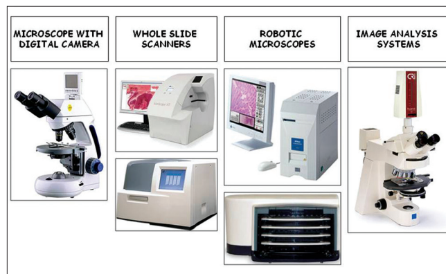
Figure 1: Input devices for creating digital images: (far left) digital camera attached via adapter to a light microscope, (middle left) whole-slide scanners showing (upper) the Aperio Scanscope XT CS Scanner, scans up to 120 slides; and (lower) the OmnyxVL4 whole-slide scanner that scans up to four slides at a time and (middle right) robotic microscopes including (upper) the Nikon CoolScope II, one glass slide scanner and (lower) the Trestle 5L50, 50 slide loaders (far right) Cambridge Research and Instrumentation (CRi) Nuance multispectral imaging (MSI) camera
