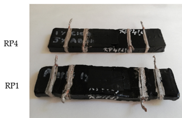
Figure 6. Image of an RP1 (1% CNT addition) specimen (lower) and an RP4 (hybrid 1% CNT + 5% graphite addition) specimen (upper) after heating tests.
