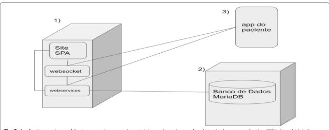
**Fig. 2** Application services architecture covering server 1, containing web services, websockets, single page application (SPA) site, which is the medical team's interface; server 2 with a MariaDB database; and the android application, which is the patient interface [19]
