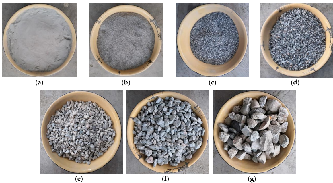
Figure 4. The aggregates screen size: (a) 0~0.075 mm, (b) 0.075~0.6 mm, (c) 0.6~2.36 mm, (d) 2.36~4.75 mm, (e) 4.75~9.5 mm, (f) 9.5~19 mm, (g) 19~31.5 mm.
