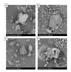
**Figure 2.** SEM images of binary systems containing bicalutamide and either PLX188 in 1:1 (**A**) and 2:1 (**B**) wt. ratio or PLX407 in 1:1 (**C**) and 2:1 (**D**) wt. ratio obtained using evaporation method.
