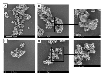
**Figure 3.** SEM images of ternary systems containing bicalutamide, PVP and either PLX188 in 4:1:1 (**A**) and 2:1:1 (**B**) wt. ratio or PLX407 in 4:1:1 (**C**) and 2:1:1 (**D**) wt. ratio obtained using spray drying.
