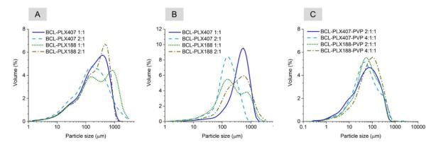
**Figure 1.** Particle size distribution of solid dispersions obtained by evaporation technique (**A**) and spray drying of binary (**B**) and ternary systems (**C**). BCL: bicalutamide; PLX: poloxamer; PVP: polyvinylpyrrolidone.
