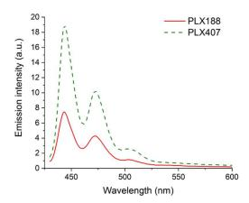
**Figure 12.** Emission spectra of perylene solubilized by either Poloxamer<sup>®</sup> 188 or Poloxamer<sup>®</sup> 407 solution ( $\lambda_{ex} = 405 \text{ nm}$ ).
