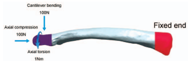
Figure 1. Diagram showing boundary and loading conditions. The sternal side was fixed in all degrees of freedom (red). The 3 loading forces were distributed over the acromial end (purple).
