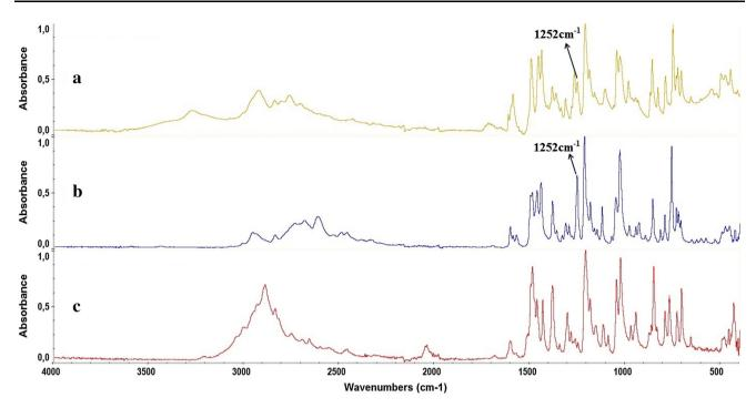
**Fig. 6** Spectral comparison showing infrared (IR) profiles obtained from the backside of a sample blotter and reference standard spectra. *Arrow* shows the decrease indicating the substitution of OCH<sub>3</sub> by OH in the 25I-NBOH. **a** Spectral profile from the back side of a blotter
