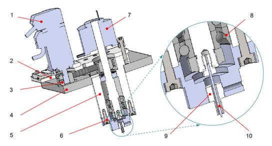
**Figure 1.** Structure diagram of integrated ER polishing tool system. (1) Driving motor, (2) Moving slide plate, (3) Synchronous pulley, (4) Support plate, (5) Outer sleeve, (6) Connection flange, (7) Conductive slip ring, (8) Deep groove ball bearing, (9) Annular electrode, (10) Tool needle.
