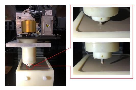
Figure 2. ER polishing equipment and flexible polishing head due to ER effect.
