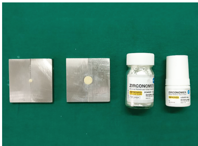
Fig. 1: Stainless steel molds with the prepared specimens
