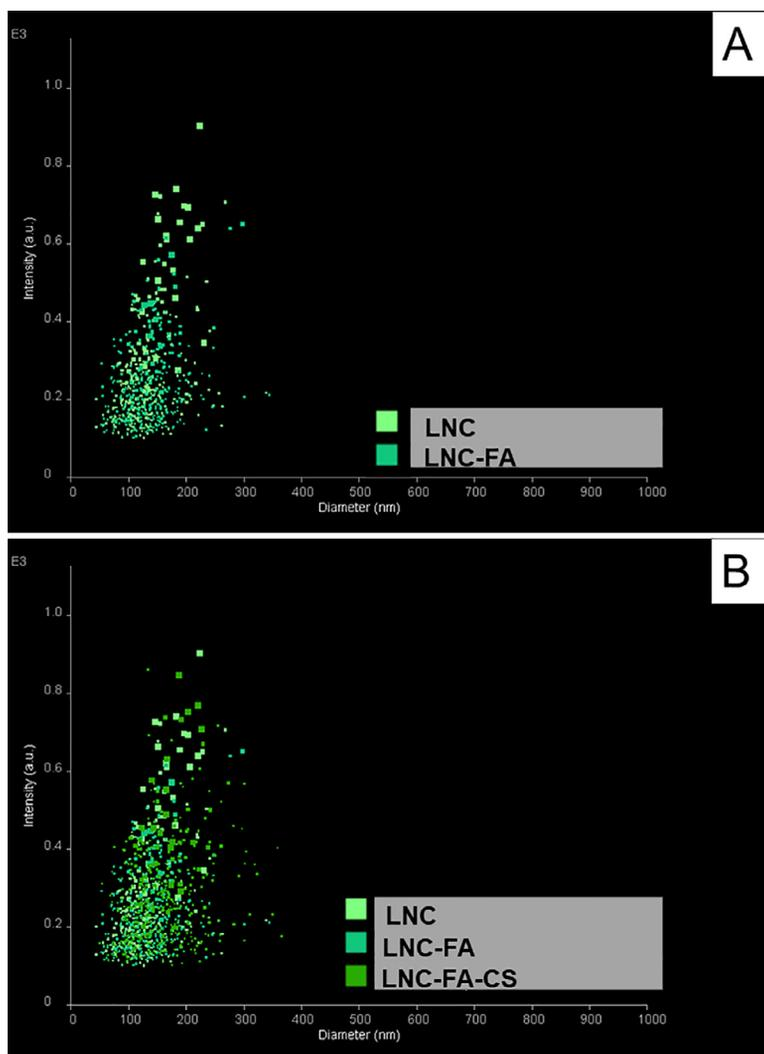
**Fig. 1.** Nanoparticle Tracking Analysis (NTA) analysis: (A) LNC: lipid-core nanocapsule and LNC-FA: fusidic acid-loaded lipid-core nanocapsule; (B) LNC: lipid-core nanocapsule and LNC-FA: fusidic acid-loaded lipid-core nanocapsule and LNC-FA-CS: chitosan-coated fusidic acid-loaded lipid-core nanocapsule.
