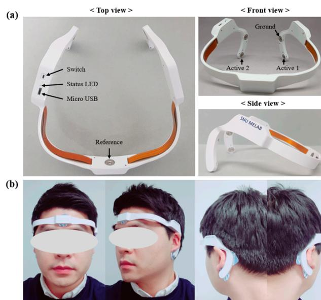
**Figure 7.** (a) The proposed wearable EEG and ECG system. (b) Photographic images of a subject wearing the system.
