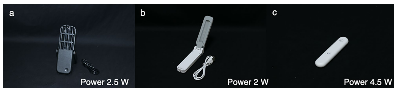
Figure 1. Three studied handheld ultraviolet germicidal irradiation surface disinfection equipment. All studied ultraviolet germicidal irradiation surface disinfection equipment were demonstrated (a; LPML1, b; LPML2, and c; LED1).
