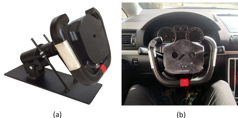
Figure 7. Two testing options—The SSW mounted on the console (a) and in the car (b).
