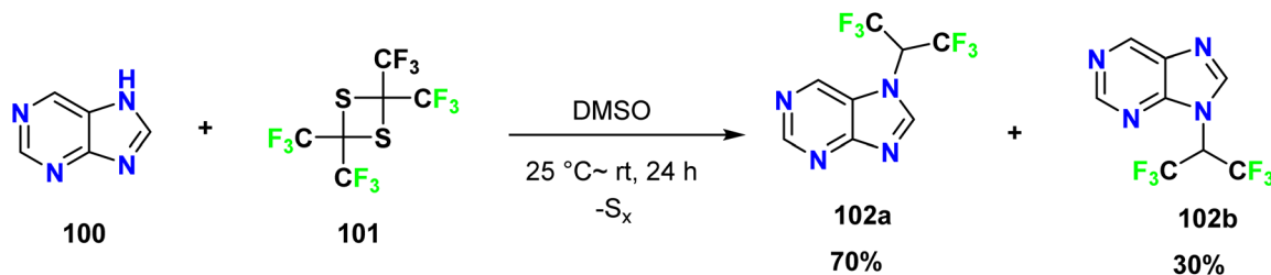
Scheme 26 Synthesis of 7- and 9-(hexafluoroisopropyl)purine derivatives 102a and 102b.
