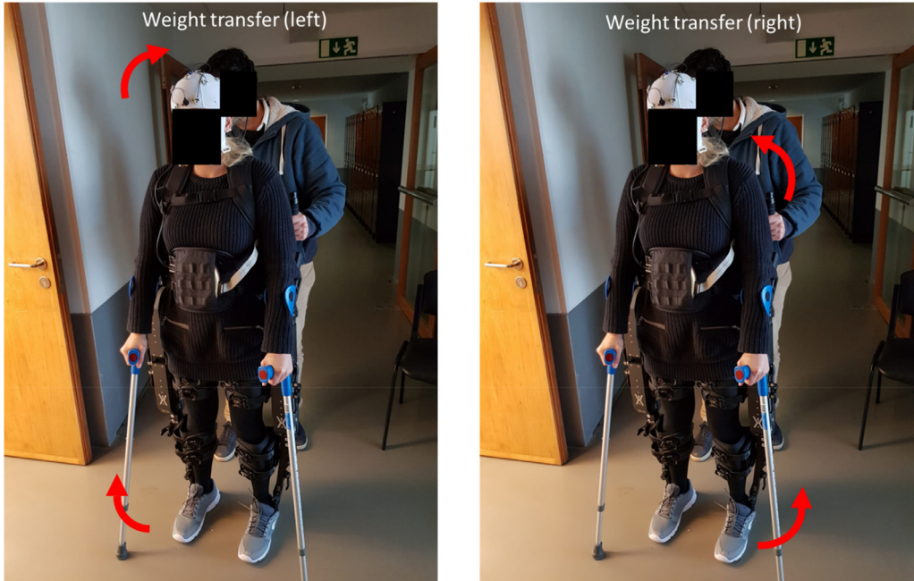
Fig. 7. Weight transfer. Before walking, the subject needs to become familiar with the weight distribution associated with the use of the exoskeleton. For this, training starts with changing weight between the left and the right leg.
