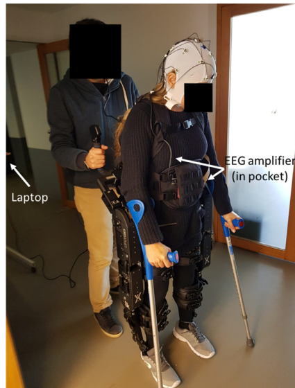
Fig. 14. EEG recordings during exoskeleton use. When recording EEG activity with the exoskeleton it is useful to have the laptop using its own battery (i.e., not using the power plug) and distant from the exoskeleton battery.
