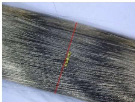
Figure 2. An image of Tenax ® -J HTS40 1420tex NiCCY provided by Toho Tenax Europe GmbH, Wuppertal, Germany. The image was taken with OneBird Smart 5M 300X USB Digital Microscope Camera Video with MicroCapture. The diameter of 6.906 mm was measured without any pretension [14].
