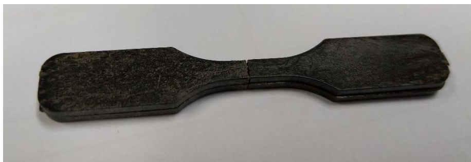
Figure 1. PBS/Lignin/PMDI/KCF composite after the tensile test.
