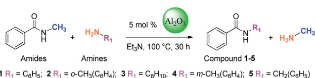
Scheme 1 Synthesis of amide derivatives 1–5.
