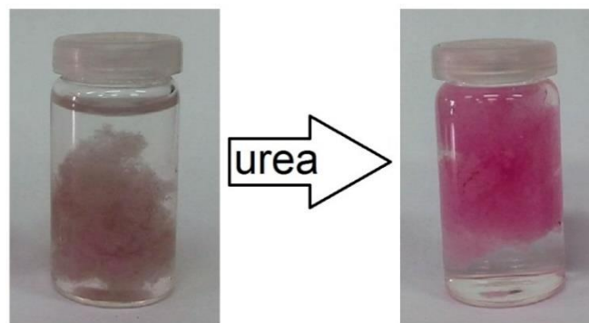
Figure 6. Biochromic color change due to releasing ammonia from reaction of urease with urea on the surface of CNF-TCFH-4.
