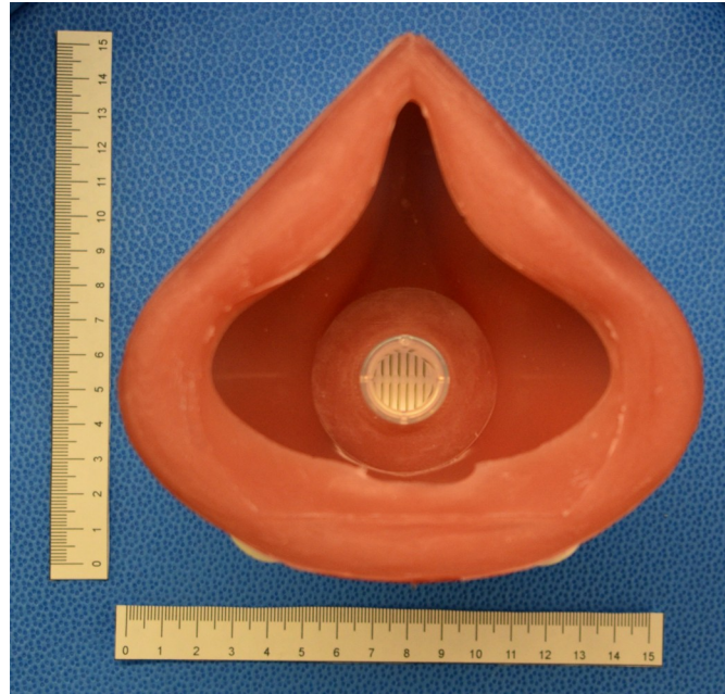
Fig 12. Inside of the silicone mask body.
