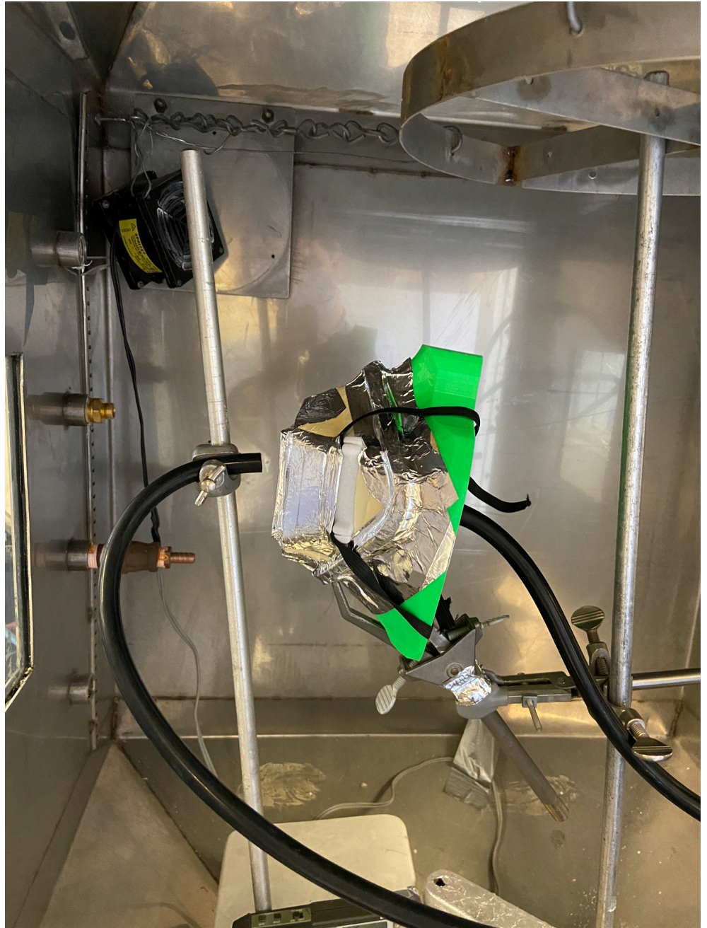
Fig 2. In-profile representation of the SFM respirator assembled on a fixture housed in the exposure chamber for filtration efficiency testing.
