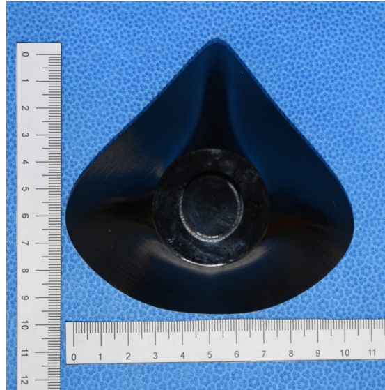
Fig 6. 3D printed mold middle component is shown.
