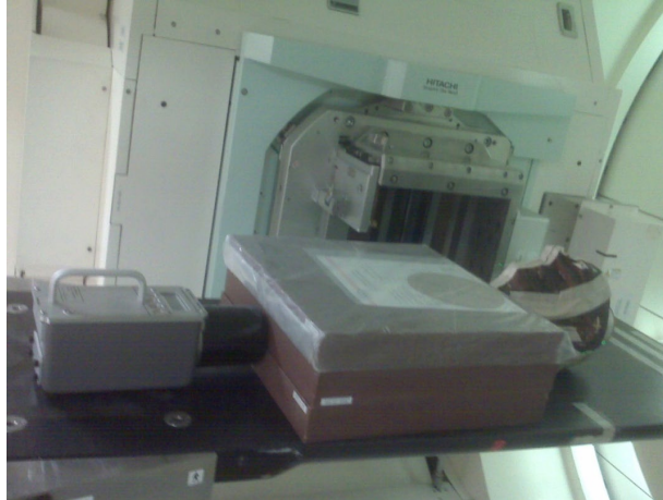
FIG. 2. Phantom used to simulate patient treatment with REM500 at the fetus representative position.
