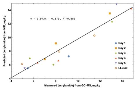
**Figure 2.** NIR acrylamide prediction. Predicted acrylamide concentration from NIR spectral data as compared to actual acrylamide concentration in mg/kg measured by GC-MS.
