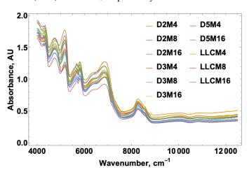
**Figure 1.** NIR spectral overlay from 4000 to 12,000 cm<sup>-1</sup> for acrylamide levels over a five-day study and fry times at 4, 8 and 16 min on each day. D = day, M = minute, LLC = LLC oil provided from a local restaurant.
