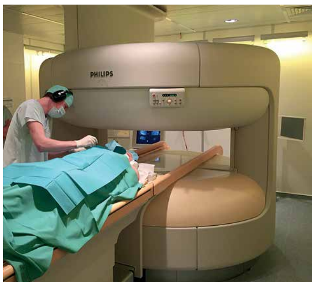
Figure 2. The open 1.0-T MRI scanner with two parallel superconducting magnet poles. The open configuration allows a direct intra-articular injection of the contrast medium. No repositioning of the patient or changing of the receiver coil was necessary
