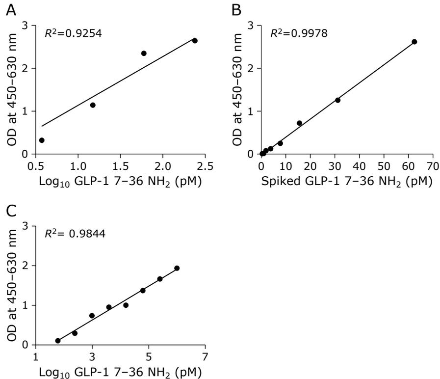
**Fig. 3.** Calibration curves of GLP-1 standards in assay (Krebs) buffer. Regression graph of GLP-1 standard [Human GLP-1 (7–36) amide] measured in Krebs buffer by the developed s-ELISAs. (A) total s-ELISA. (B) sensitive active s-ELISA. (C) Wide-range active s-ELISA. Points are means from triplicate determinations.
