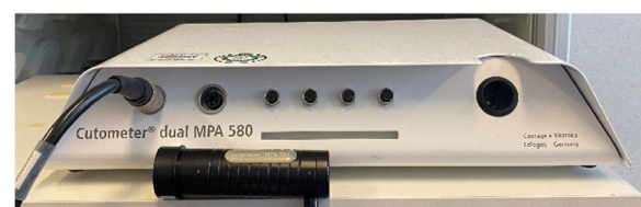
Fig. 6 The Cutometer measures scar mechanics retraction, elasticity, viscoelasticity, and maximum extension by inducing negative pressure on scar tissue (Cutometer Skin Elasticity Meter Dual MPA 580 ® Courage and Khazaka GmbH, Cologne, Germany)
