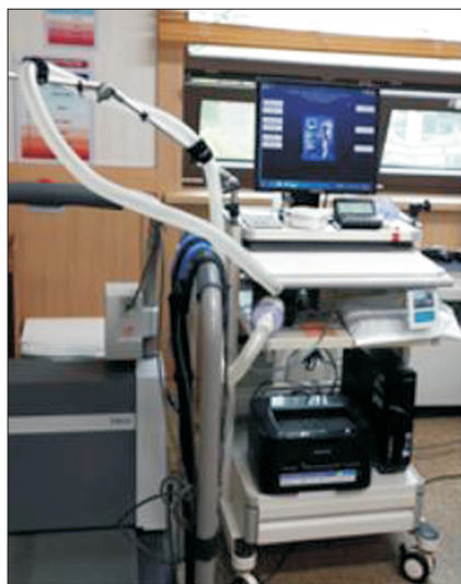
Fig. 2. The TrueOne 2400 metabolic system (Parvo Medics, Sandy, UT, USA), which measures the cardiometabolic parameters.
