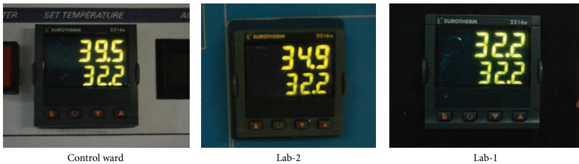
FIGURE 7: Incubator performance on typical extreme hot day of October 17, 2012. Readout top (actual chamber temperature) and bottom (set-point).
