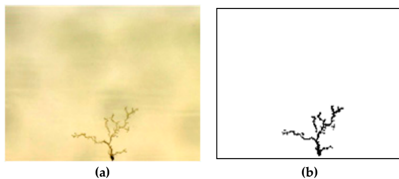
Figure 6. Example of electrical tree image binarization processing. (a) Electrical tree original image, (b) Electrical tree after image binarization processing.
