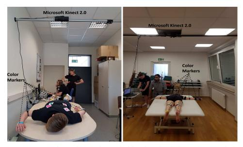
**Figure 2.** Camera setup during the recording in the lab (**left**) and in the hospital (**right**). The camera (Microsoft Kinect 2.0) was hooked with the help of an autopole at the height of 2 m with an angle of 90° from the table surface where the patient is lying for therapy.
