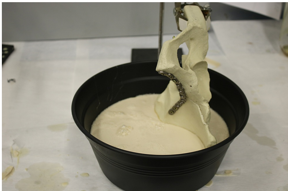
FIGURE 7: Pelvis fixed at the desired angle
