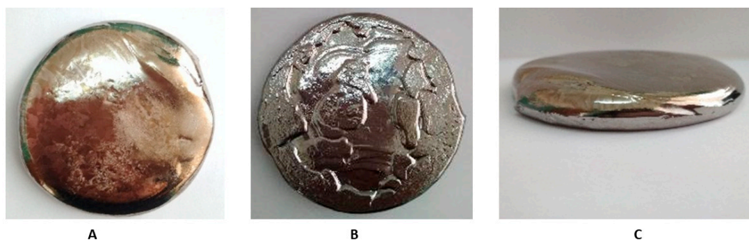
Figure 1. Zr-Ti-Nb ingot after arc melting—upper (A), lower (B), and lateral (C) view.
