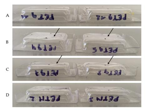
**Figure 13.** PETg trays exposed to hot-fill temperatures of 75 °C (**A**), 85 °C (**B**) and 95 °C (**C**), and PETM trays exposed to hot-fill temperatures of 95 °C (**D**).
