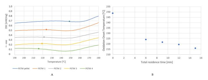
**Figure 5.** (**A**) DSC signal of the STA analysis of the PETM residence time samples (Table 1) for the determination of the oxidation onset temperature (dots). (**B**) Oxidation onset temperature vs. residence time for PETM samples.
