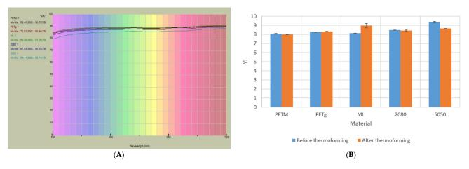
**Figure 11.** (**A**) VIS spectrum of sheets and trays. (**B**) Yellowness index values of the sheets (blue) and thermoformed trays (orange) (Table 2).
