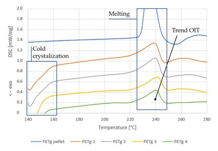
**Figure 6.** DSC curves of the STA analyses of the PETg residence time samples, extruded with the HAAKE Minilab twin-screw extruder, for the determination of the oxidation initiation temperature.
