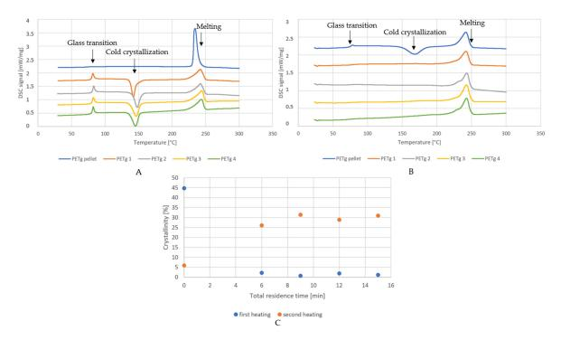
**Figure 4.** DSC curves of the first (**A**) and second (**B**) heating run of the PETg samples. Crystallinity of the PETg residence time samples vs. total residence time (**C**) (Table 1).
