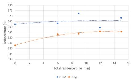
**Figure 7.** Temperature at which the residence time sample, extruded with the HAAKE Minilab twin-screw extruder, lost 5% of its mass, with the dashed lines as a guide for the eye.
