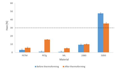
**Figure 10.** Haze of the sheets, extruded with the Labtech co-extrusion unit, and the thermoformed trays.
