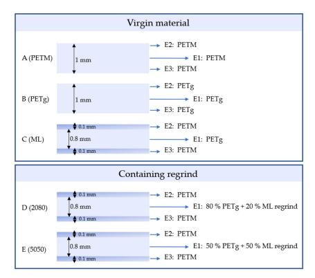
**Figure 1.** Composition of the produced multilayer sheets in this work, with a relative layer thickness distribution of 10/80/10. (**A**,**B**): pure sheets (PETM, PETg), (**C**): multilayer (ML), (**D**,**E**): the multilayer containing 20% regrind (2080) and 50% (5050) regrind in the middle layer.
