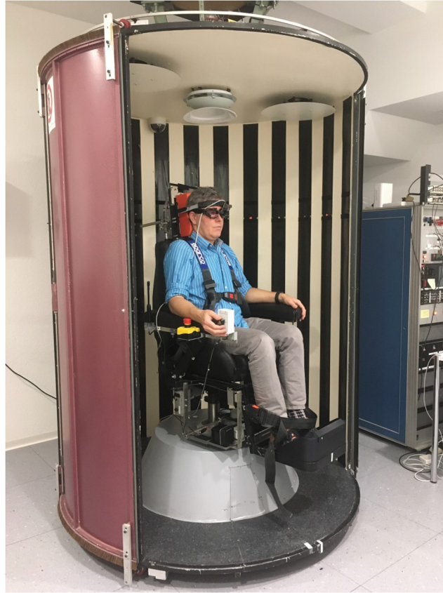
Fig 1. Experimental set up with motorized chair and drum that could rotate independently from each other. During the test the surrounding drum was closed and rotating around the stationary chair.
