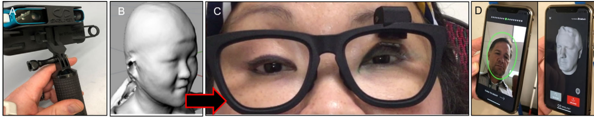
Figure 4. Craniofacial 3-D scanning and printing methods. (A) Structure sensor attachment for iPhone 8. (B) Craniofacial scan produced for participant 5 using (A). (C) Custom MLP frame generated for participant 5 from (B). (D) The sensor attachment is no longer needed for iPhone models X and above.
